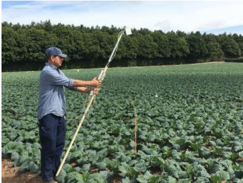
Figure 55. Use of handheld CropScan sensor to measure reflectance from the crop canopy
