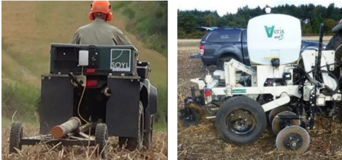
Figure 2. Measuring soil electrical conductivity using a non-contact EMI scanner (left) and a contact Veris MSP3 EC scanner
