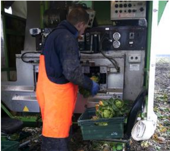
Harvest machine strips sprouts from stalk
